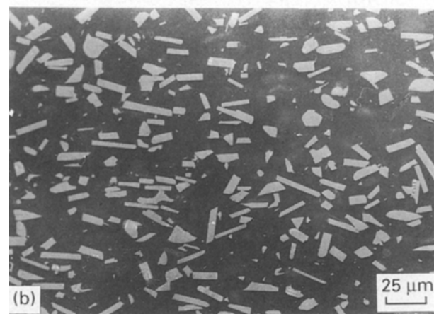
Figure 9 (a, b) Optical micrographs of Al 2 O 3 /20 vol% SiC platelet composites obtained by hot pressing at 1500 °C for 1 h and 50 MPa in argon.
